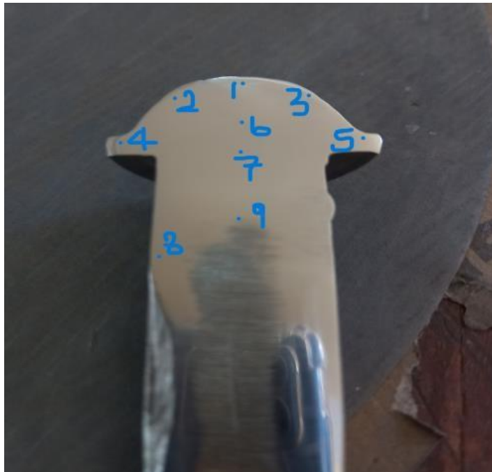
Figure 4 – Hardness measuring points of specimen
