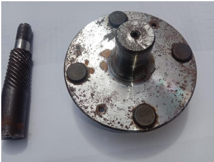
Figure 1 - a typical front wheel axle that has been broken while in operation
